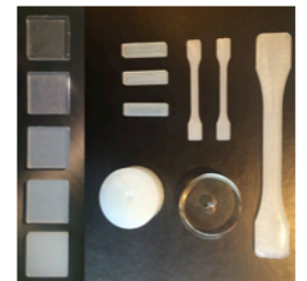
Nanosferix composite material test articles: polyurethane (left) and epoxy (right). Loading of Nanosferix particles varies from 0.01 to 0.1 wt %.
